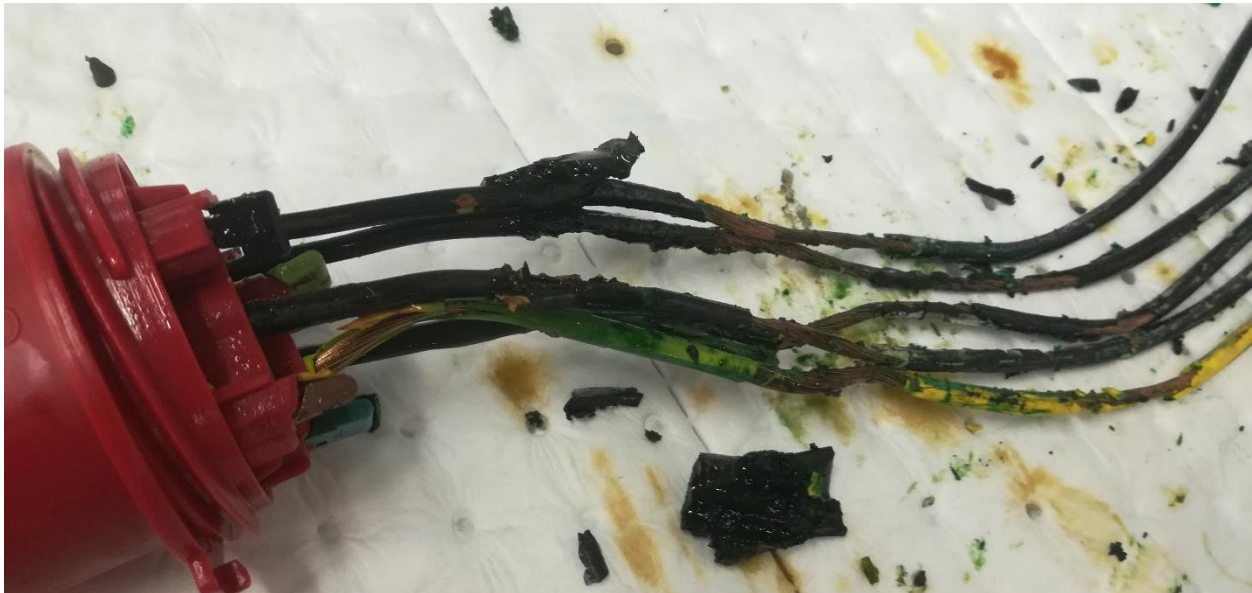
Figure 1: Power cable after wicking oil from oil bath. 1
